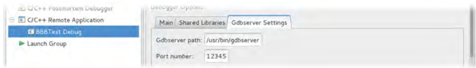
Figure 7-9: Setting the BBB gdbserver port
